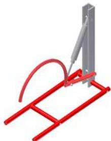
The fourth design was made between the two competitions used a small PVC hook actuated by a pneumatic cylinder to clamp down on the tube. Since we could not add this pump system to the robot, this was unusable.
