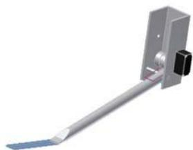
The original design was comprised of an actuated hook attached to the end of a rotating arm. The hook would start flat, and could then slide under the tube. A motor would then pull on a string which would, in turn, lift a flap of plastic, holding the tube in place. The arm could then rotate to whatever height was required to place the tube on the rack.
