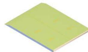
The final design utilized aluminum honeycomb, which is usually found in aircraft flooring. This light and durable material proved to be exactly what we needed, as it withstood the weight of other robots while freeing up some much-needed weight.
